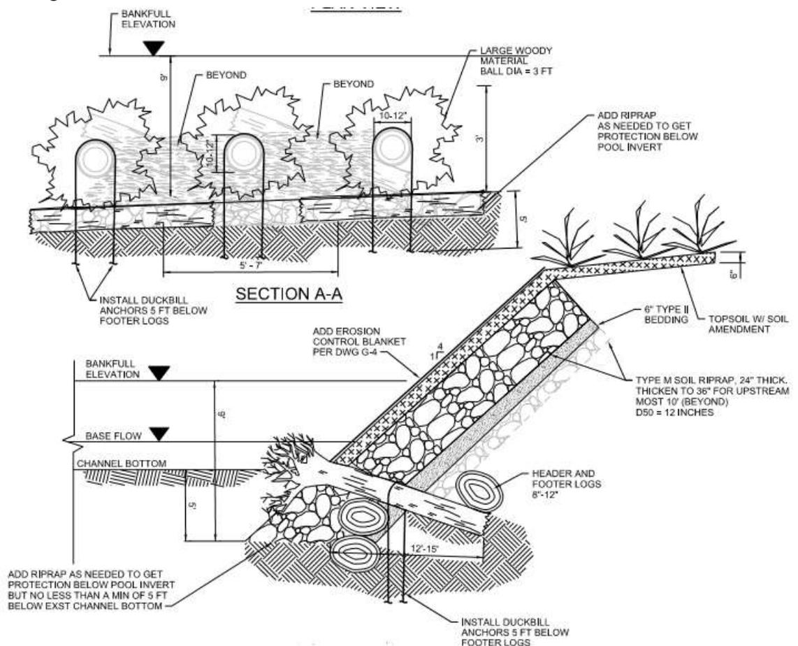
Figure 7: Woody toe and bank stabilization
